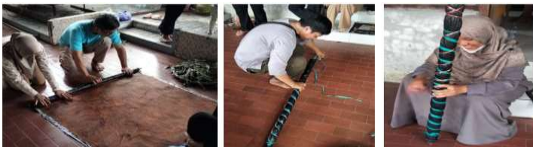
Figure 6. The Process of Rolling Fabric with a Roll as Part of the APEc_3 Tool
